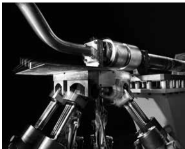
Fig. 2.5 Vibration test bench for simulation of complex application conditions
