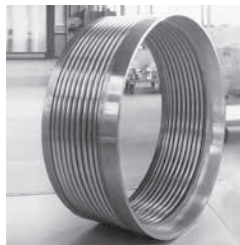
Fig. 8.6 Axial expansion joint made of Alloy 825 for heat exchanger (DN 1200/PN 40)
