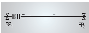
Fig. 9.5 Asymmetrical arrangement of the expansion joint. Frictional force acting on one anchor.
