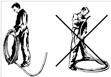
Fig. 4.7.1 Proper (left) and incorrect handling (right) of hose assemblies
