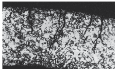
Fig. 7.4 Transgranular stress corrosion cracking on a cold strip made of austenitic steel. Sectional view (50-fold enlargement)
