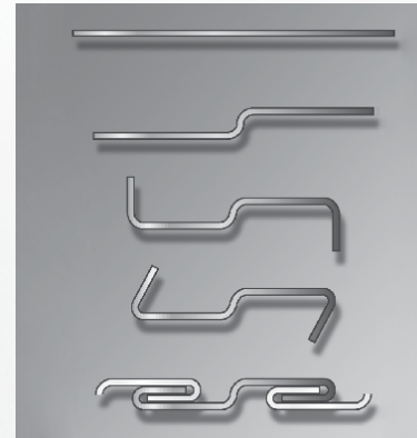
Fig. 2.6.1 Profiling and integration of the cold rolled strip (schematic, left) and production of stripwound hoses (right)
