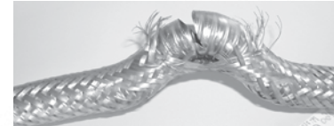
Fig. 4.1.2 Braiding failure and resulting ruptured hose
