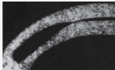
Fig. 7.6 Crevice corrosion on a cold strip made from austenitic steel. Sectional view (50-fold enlargement)
