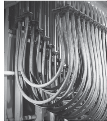
Fig. 3.1.8 Metal hoses in a multiple press.
